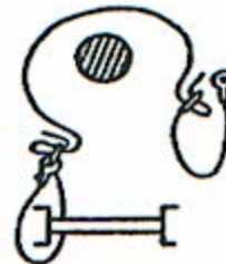
STEP 1 Place the strap between the fourth and fifth rungs with the snaps facing outward.
