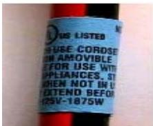
Could you plug a 150 watt lamp, a 60 watt lamp, and an appliance which uses 10 amps at 125 volts into an extension cord rated **15 amps/1875 watts**? Let's do the math: 10 amps x 125 volts = 1250 watts. Add the wattage of all the appliances together:
