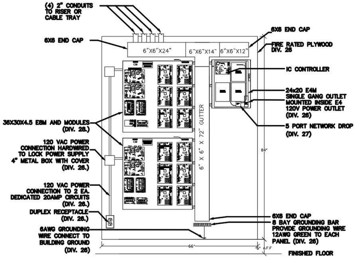
Figure 2 - Example of Typical CAAMS Backboard
