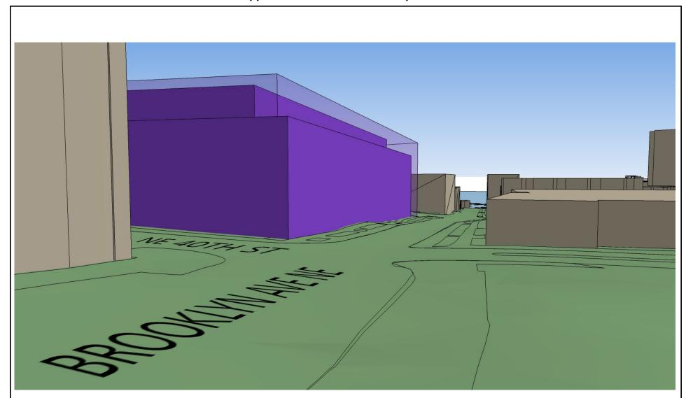
Note: This illustration is intended to represent a conceptual plan and massing for the Population Health Facility under Alternative 1 and is not intended to represent the specific project design. The conceptual massing is indicated in the figures in dark/solid purple and the CMP-Seattle 2003 building envelope is indicated by a lighter/translucent purple.
