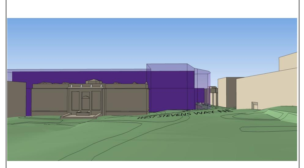
Note: This illustration is intended to represent a conceptual plan and massing for the Population Health Facility under Alternative 2 and is not intended to represent the specific project design. The conceptual massing is indicated in the figures in dark/solid purple and the CMP-Seattle 2003 building envelope is indicated by a lighter/translucent purple.
