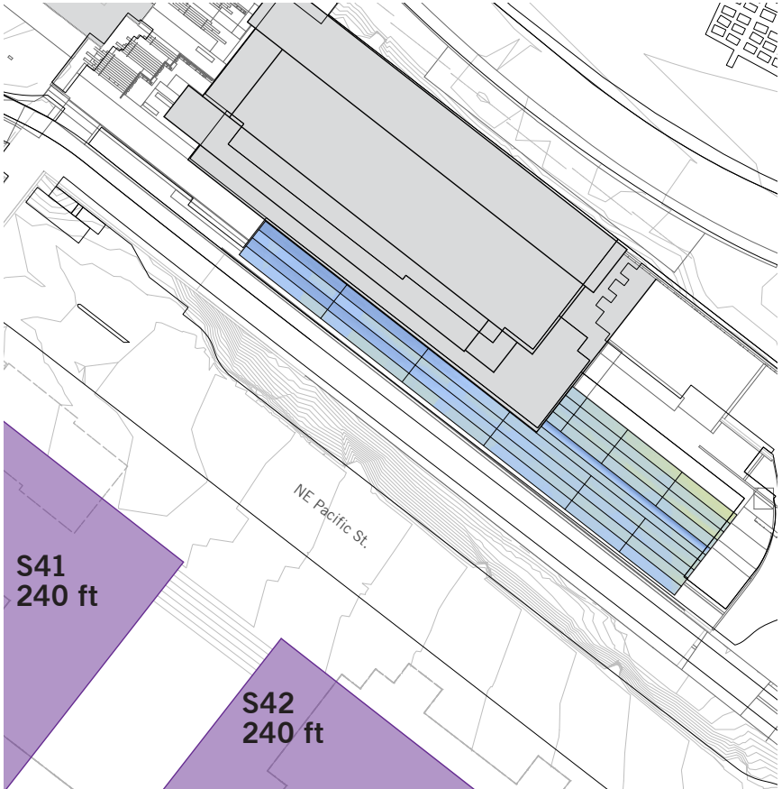
Figure 3.3 January Cumulative Incident Solar Radiation (kWh/m 2 ) - All South campus buildings at 240 ft height
