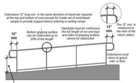
Extensions with a leading edge 27° high max, can extend any amount from posts. Those with a leading edge higher than 27° are limited to a 12° protrusion from posts (§307.3). The sloping portion of handrails are not required to comply with requirements for protructing objects.
