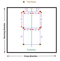
Figure 5-1 - Walkway Local Flatness Measurement for Running and Cross Slopes
