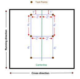
Figure 5-5 - Ramp Local Flatness Measurement for Running and cross Slopes – Profile View
