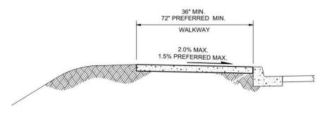
Figure 4-1 - Walkway Width and Cross Slope
