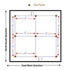
Figure 5-6 - Ramp Local Flatness Measurement for Slopes (Architectural Research Consulting, 2011)
