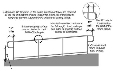
Extensions with a leading edge 27" high max. can extend any amount from posts. Those with a leading edge higher than 27" are limited to a 12" protrusion from posts (§307.3). The sloping portion of handrails are not required to comply with requirements for protruding objects.
