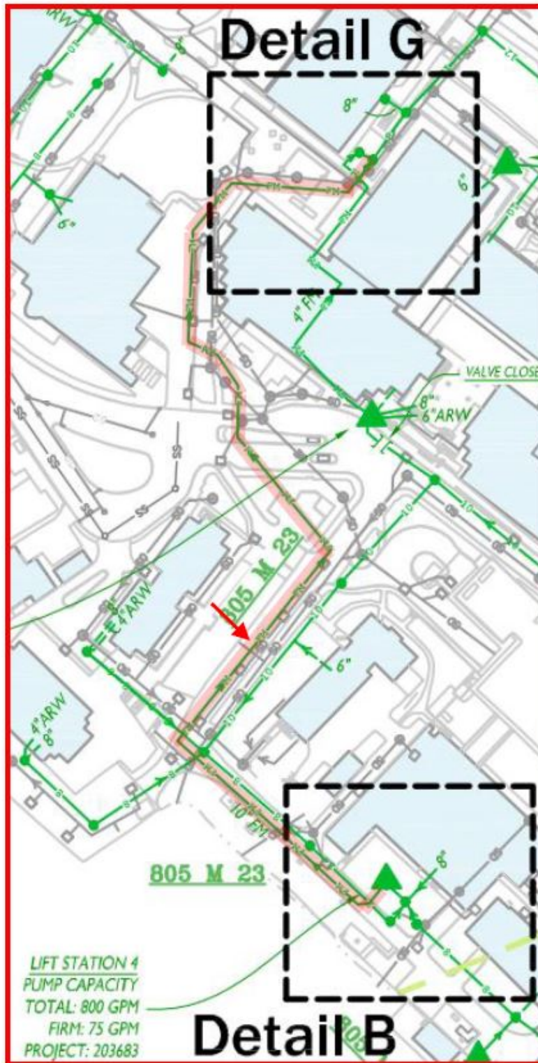
Figure 2 - Force main highlighted in pale red. Approximate leak location denoted by red arrow.
