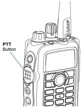
While a call is in progress, the PTT button allows the radio to transmit to other radios in the call.
